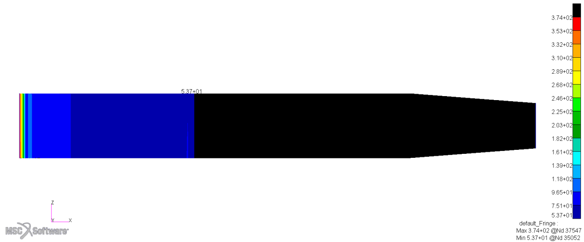
Figure 2-10 Contact stresses of the extension
