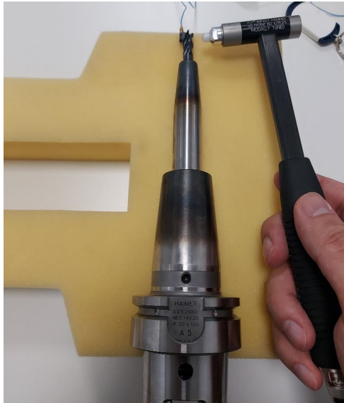
Figure 4-3 Modal testing of holder-extension assembly at the tip of the tool
