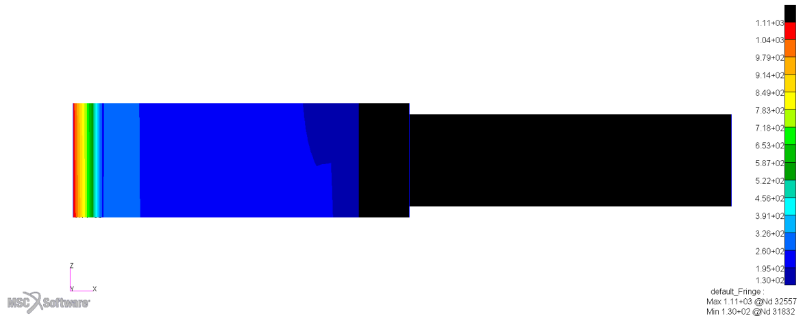
Figure 2-11 Contact stresses of the tool
